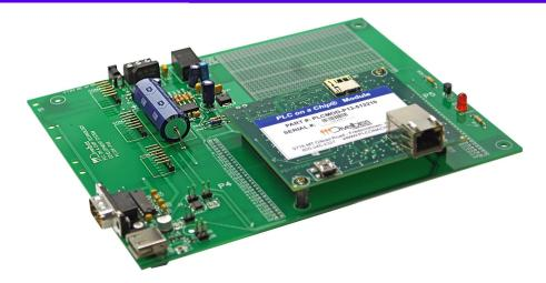
The P-Series PLC on a Chip Development Kit is a development tool for the P-Series PLC on a Chip. Included is the complete library of documentation required to apply P-Series PLC on Chip at the module and integrated circuit level, the development board and the EZ LADDER Toolkit software.
