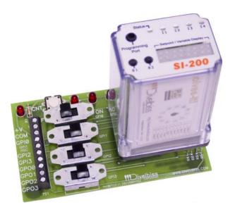
The Trainer/Simulator boards are intended for use by industry and educators. Industrial use includes testing both proof of concept programming as well as final hardware programming on the bench rather than the machine to eliminate costly machine down time. Program development for Solves-It! plug-in PLCs or other PLC on a Chip® based products is greatly simplified. Other uses include continuing education for shop maintenance and/or technical personnel and initial training for new hires.
