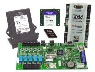
OptiCAN is a Divelbiss proprietary CAN (Controller Area Network) protocol that provides a commuication link between Divelbiss OptiCAN enabled controllers and other OptiCAN enabled devices such as I/O modules and controllers. The Divelbiss OptiCAN network supports up to 64 nodes (devices) and is register based. Each node supports up to 256 registers and communication can be triggered based on time or on an event.
