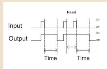
The operation of the [Time Delay on Pick Up or TDPU](#) function is somewhat the opposite of the TDDO. The preset timer begins as the trigger is applied i.e. on the rising edge of the signal. After the timer elapses, the output will energize. The output will remain energized until the input signal is removed. The timer will reset if the input signal is removed. A typical
