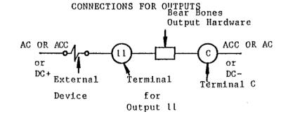
NOTE: For output connections AC and ACC may be interchanged. See sheet 8 for additional connection comments.
