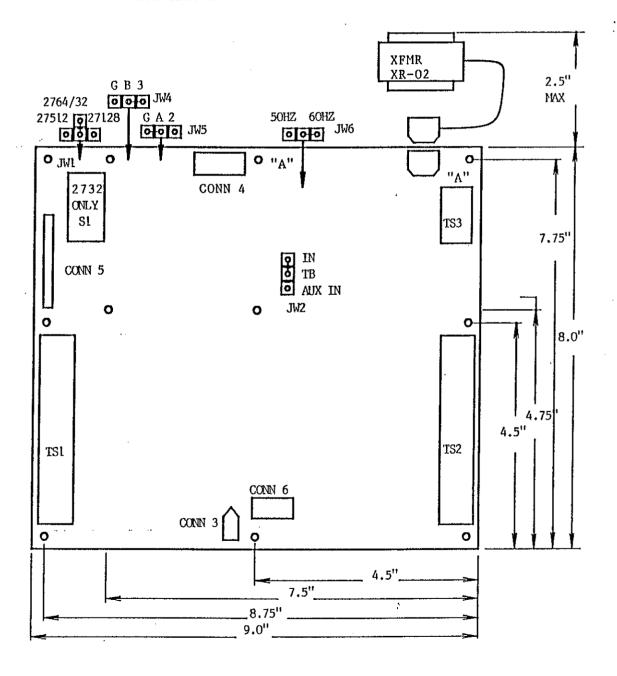
CAUTION: Connect transformer before wiring TS3.
