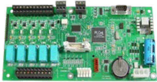
ICM-EBB-700 Programmable Logic Controller
